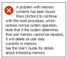
If this message appears, press Action, which starts the reset procedure. Note, however, that you may not be able to perform a reset if memory contents are corrupted. In such a case, you will have to perform a full reset, which is described on the next page.
